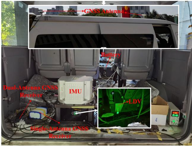
Fig. 5. Installation diagram of the experimental system.
